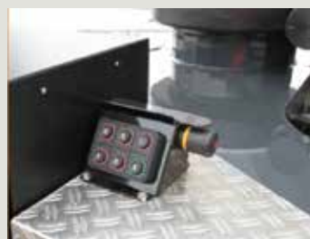
Chassis outrigger controls
